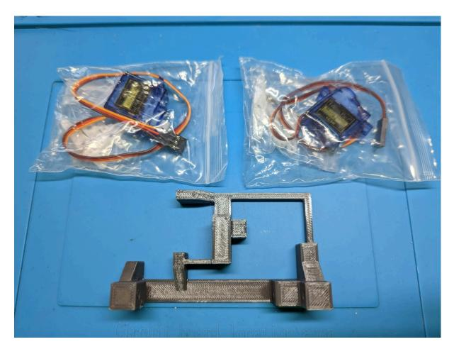
The servos usually come with three screws and a few adapters for RC vehicles. We don't need those adapters. The two larger screws are used to fix it to the laser cage. The small one is for the gear.
