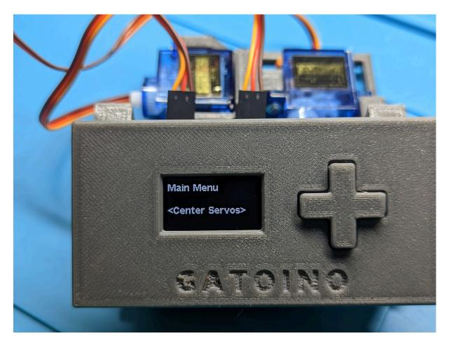
Before we add the mirrors we need to center the servos in order to ensure a maximum freedom of movement in all directions.
