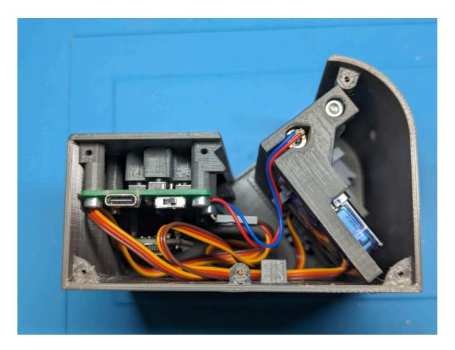
The backside of the case features a "bridge" which is meant to route the serve cables through. This is to prevent them from contact with the moving gears. Route those two cables from top to bottom first (connectors in direction of the case bottom).
