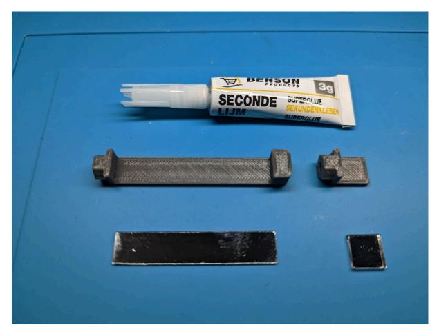
The mirrors are glued to their respective axis. It's easiest to use superglue. Make sure the mirror doesn't have any foil on its back. Some come with adhesive tape but I still recommend adding glue since that tape doesn't bond that well with printed parts. Make sure the glue is fully cured before you proceed.
